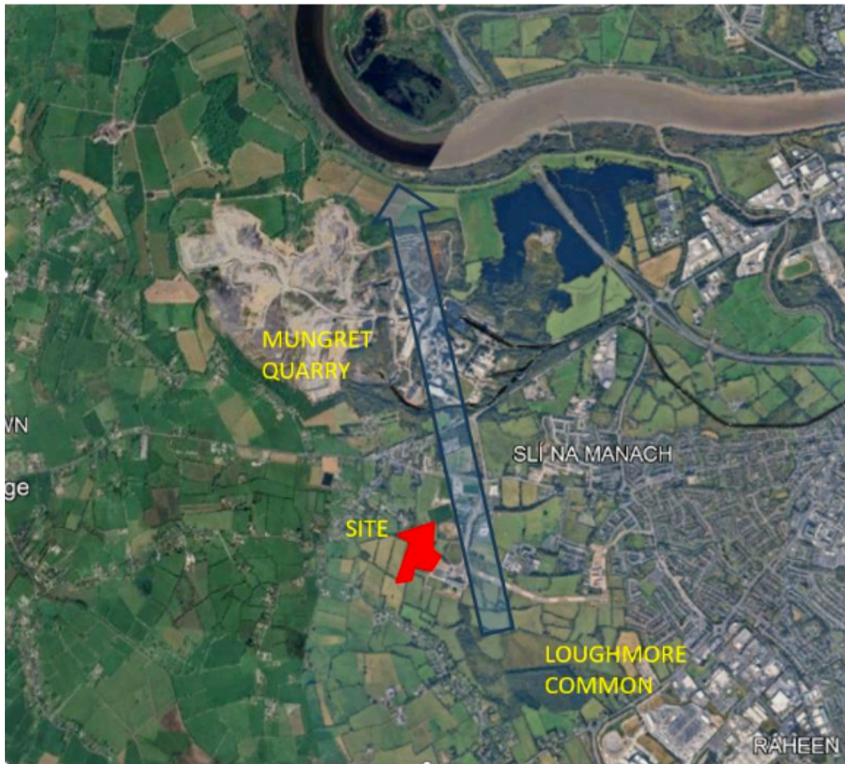
Figure 6. Groundwater Flow Direction
